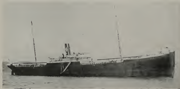
The ARAB (later the M.S. Dollar) the first vessel to be converted from coal to oil.
